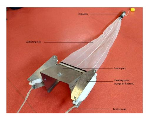
FIGURE 2 | Picture of a Manta net sampling device.
