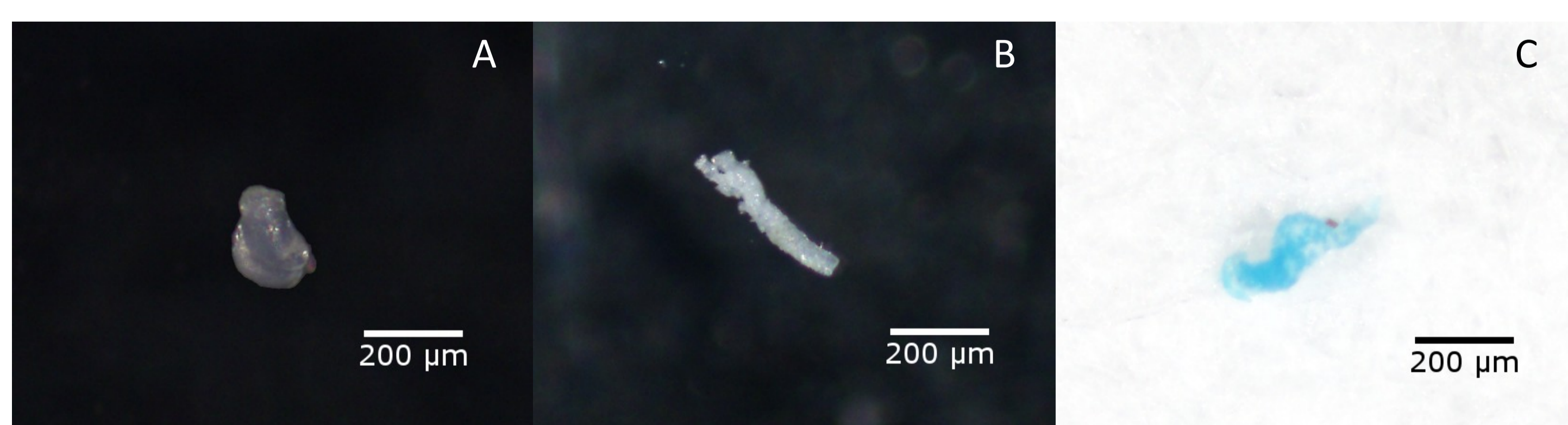
Figure 2: Pictures of particles recovered from mussels and cockles samples successfully identified (A-B) and partially (C) by Raman spectroscopy.
