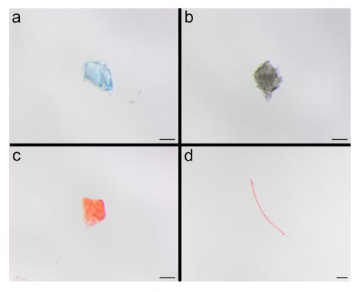
**Fig. 1.** Pictures of microplastics fragments and fiber used to fill the capsules including: (a) blue high-density polyethylene (HDPE), (b) gray polypropylene (PP), (c) red polystyrene (PS) fragments and (d) red polyester (PES) fiber. Black bars at the right bottom of each picture represents a length of 100 µm.
