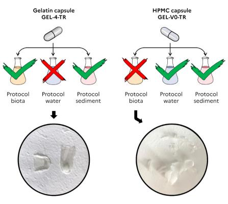
Fig. 2. Main results obtained after filtration of solutions containing capsules from the three tested protocols. GEL-4-TR capsules were not efficiently dissolved with water and GET-V0-TR capsules were not efficiently dissolved with 10% (w/w) KOH.
