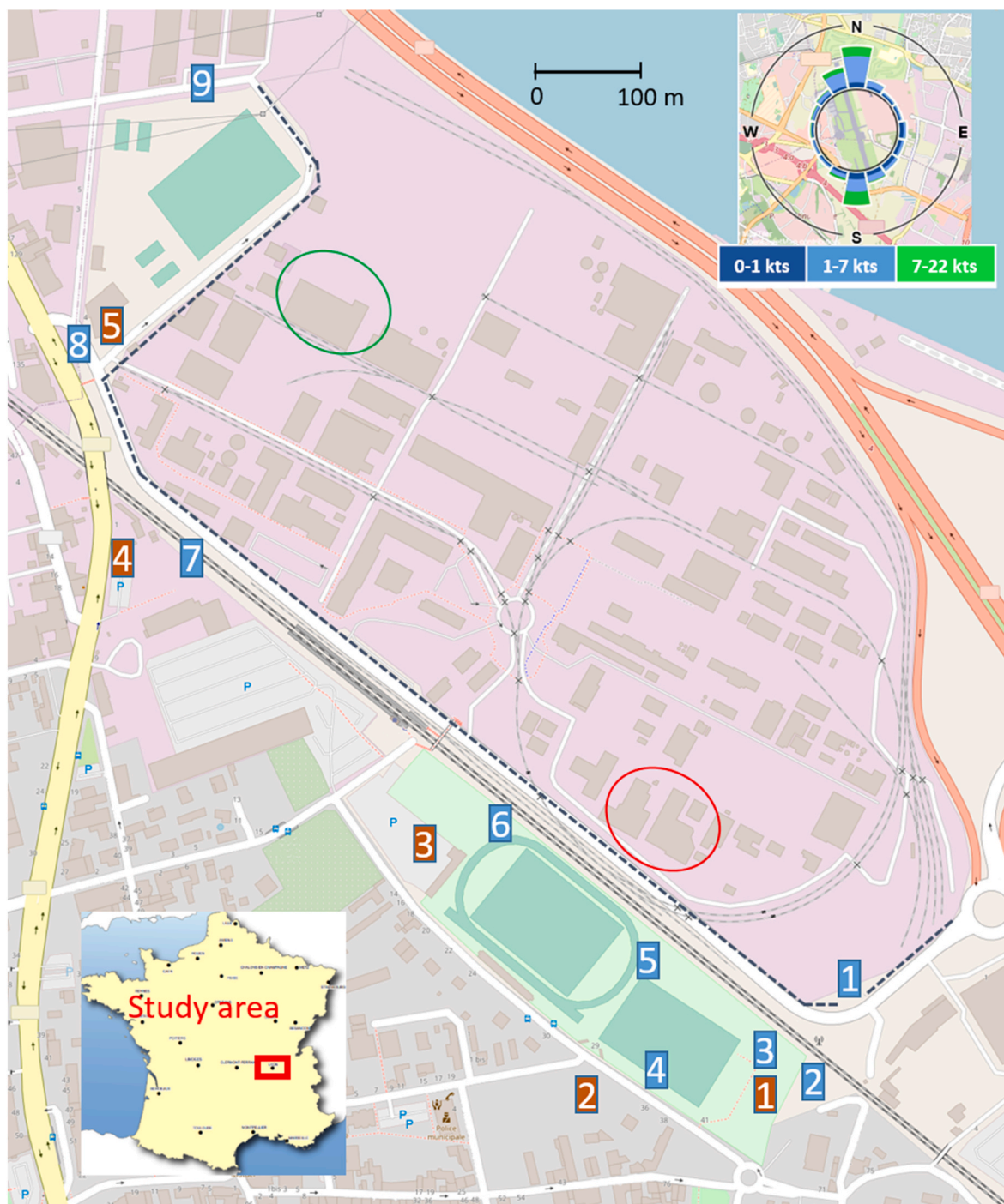
Fig. 1. Soil (blue squares) and dust (orange squares) sampling locations. The wind rose at the top right represents the annual average in knots (kts) for prevailing wind based on data from a measuring station 9.3 km east of the industrial park. The PVDF production unit is indicated by a red circle, the fluoroelastomer unit by a green one, and the industrial park's perimeter fence by a black dotted line.
