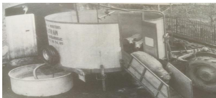
Figure 12 : Illustration de la douche Solitram (Pâtre 1985)
