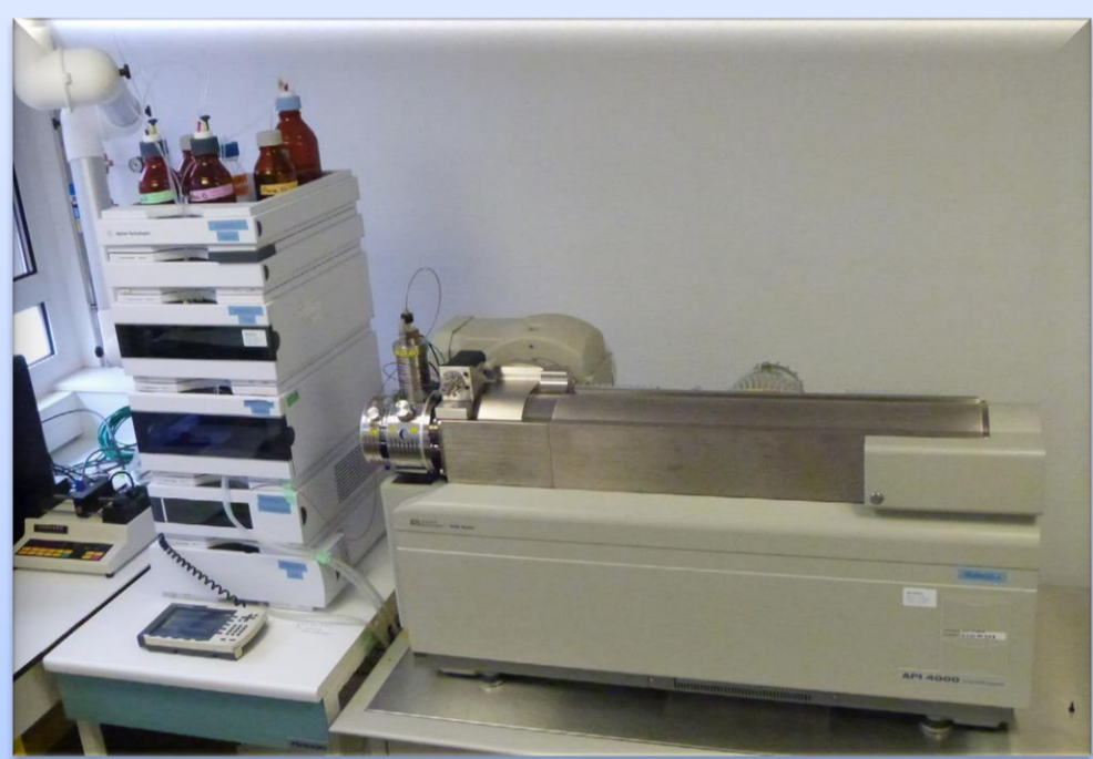
LC Instrument: Agilent 1200 series MS Instrument: AB Sciex API 4000
